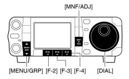
While adjusting the manual notch filter, noise may be heard. This comes from the DSP unit and does not indicate an equipment malfunction.
